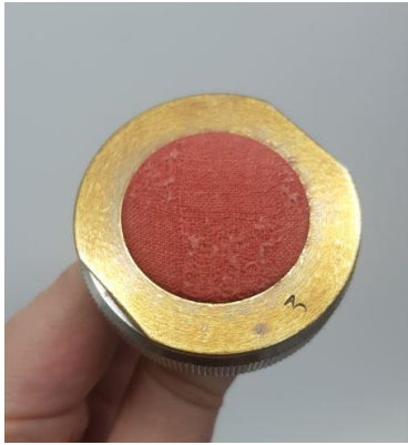
Fig. 16. Holder of Martindale abrasion and pilling tester
