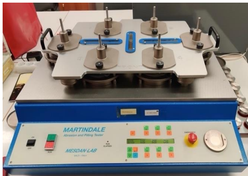
Fig. 15. Martindale abrasion and pilling tester MESDAN-LAB, Code 2561E (SDL AT-LAS, London, England)
