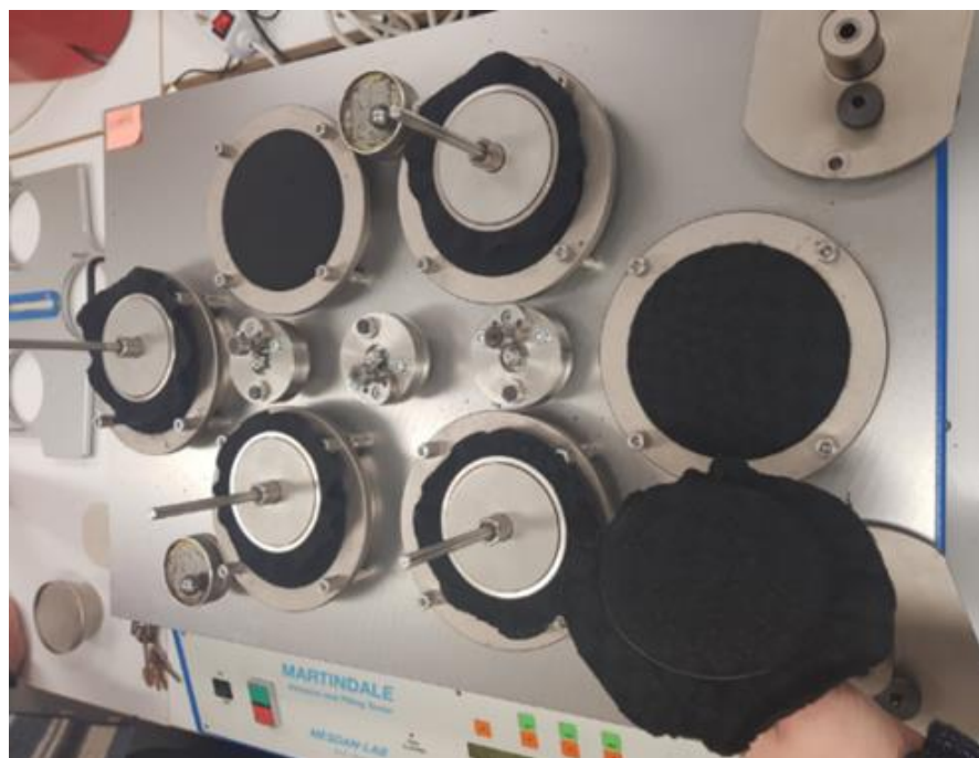
Fig. 14. Sample pairs on the holders and pilling tables
