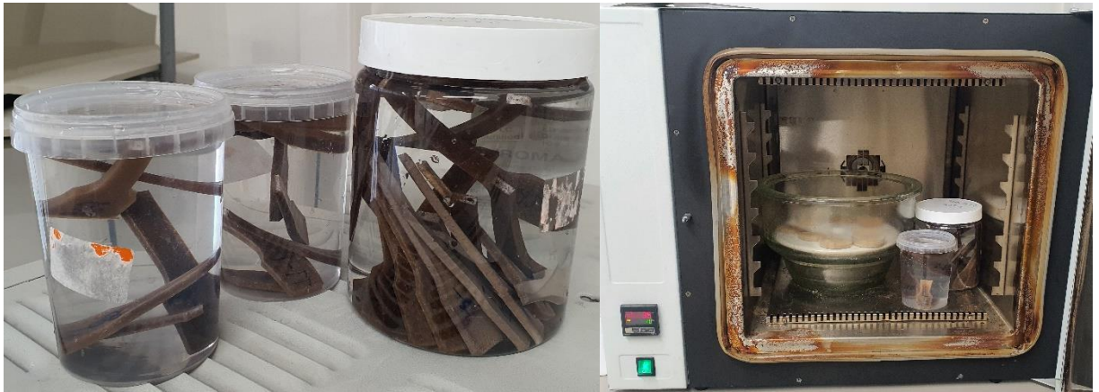
Fig. 12. Samples of PP composites placed in the oven for water absorption analysis
