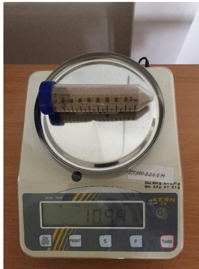
Fig. 13. Determination of bulk density of filler particles
