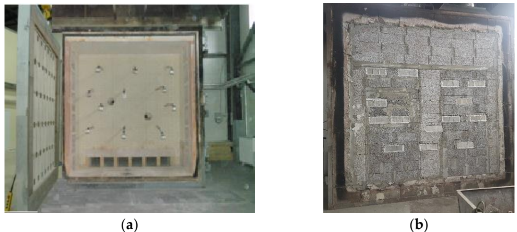
Figure 3. The oven for fire resistance test. Open test wall (a) and close test wall with constructed concrete samples in it (b).
