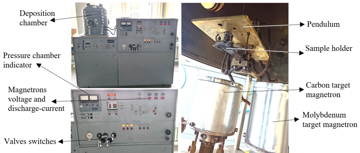
Figure 1. The photo of magnetron deposition system, control panel with the main elements (left) and deposition chamber (right).
