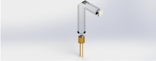
Fig. 7 Light guide based optical device CAD model
