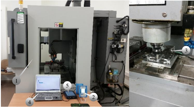
Fig. 2 Experimental setup of the friction stir welding experiments: 1 – machining centre LEADWELL V-20; 2 – “Kistler” amplifier; 3 – “Kistler” force sensor; 4 – computer; 5 – oscilloscope
