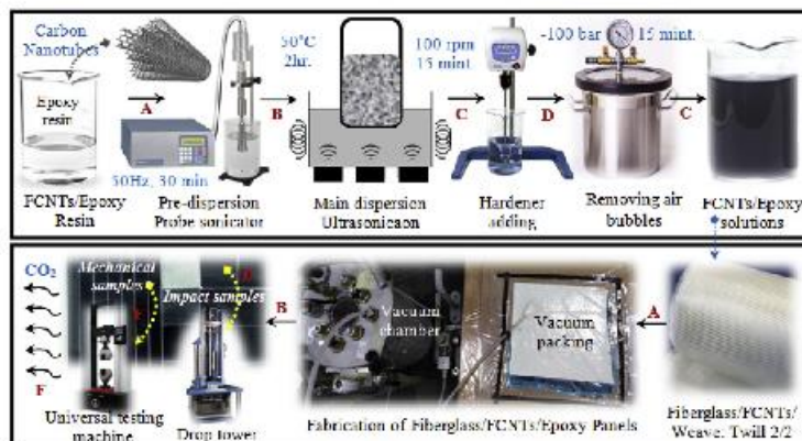
Fig. 2. Fiberglass/FCNTs/epoxy laminate nanocomposite panels - preparation and characterization flowchart.
