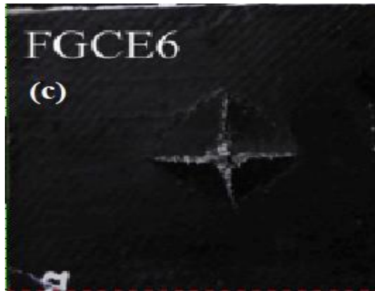
Fig. 2.5. Impact performance assessment from the numerical mode: (a) load displacement curve, (b) shear stress distribution from the model, (c) failure profile during the experimental impact
