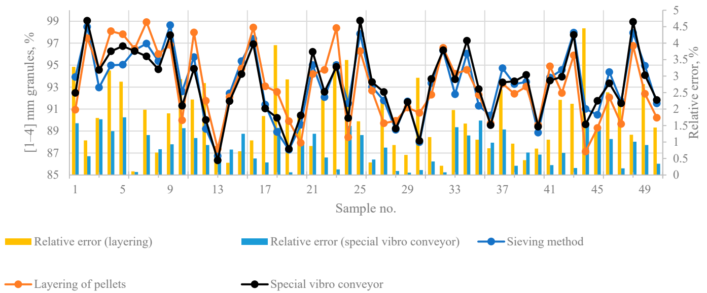
Figure 9. Comparison of granulometric composition results using a special vibroconveyor prototype.
