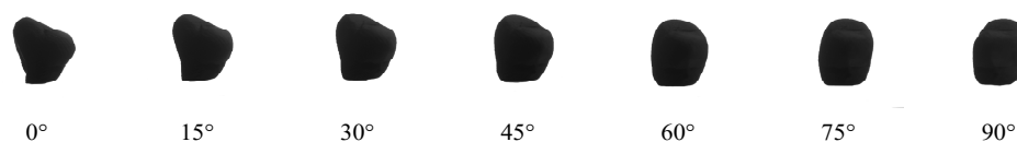
Figure 5. Scanning of particles at different angles relative to their falling plane.
