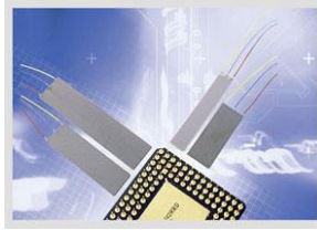
1.11 fig. Multilayer PICMA company bending piezoelectric actuator
