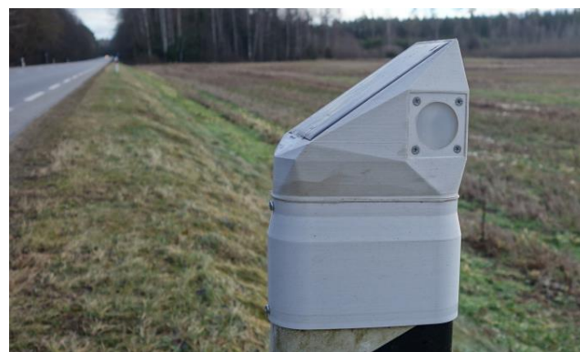
Figure 12. The second-generation DSN mounted on a roadside-marker post.
