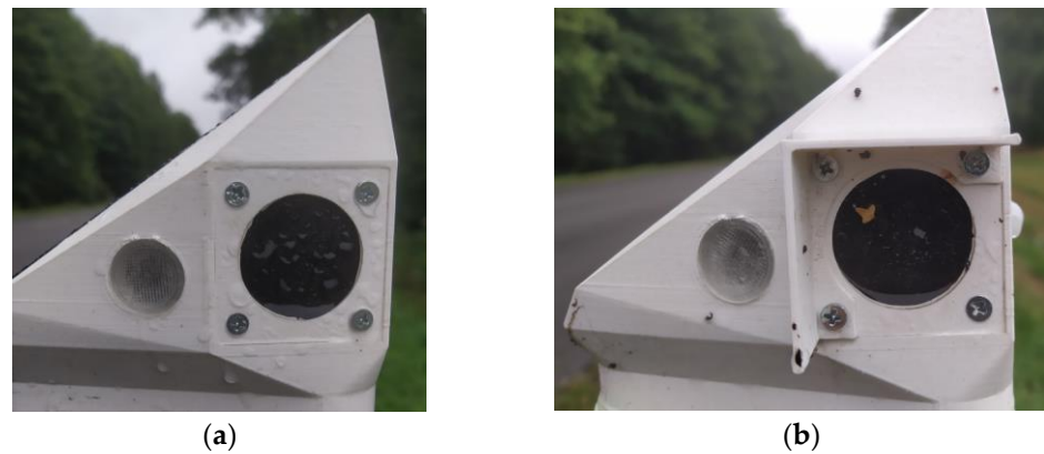
Figure 11. Photos of the installed first generation of DSN nodes with various types of optical contamination: (a) Raindrops on the sensor opening; (b) Organic particles and raindrops on the sensor opening with the installed canopy.
