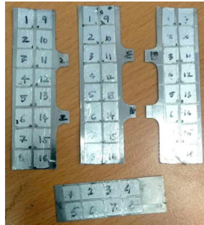
Figure 3. The aluminum foil was glued to the steel core to measure the quality of the glue.
