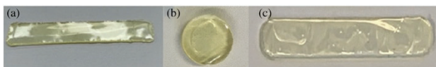
FIGURE 2 Specimens used for tension (a), compression (b), and bending (c) tests. [Color figure can be viewed at wileyonlinelibrary.com ]
