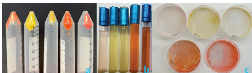
Figure 2. Pigment extraction (a – biomass of pigmented microorganisms, b – extracted pigments, c – dried pigments).
