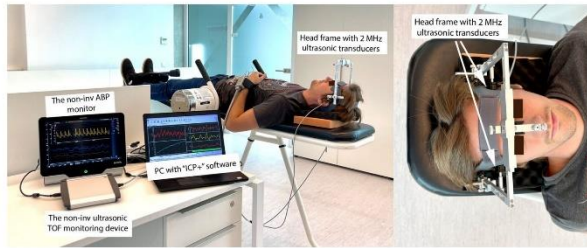
Figure A1. The CA monitoring setup includes the noninvasive ultrasonic TOF monitoring device with the head frame, noninvasive blood pressure monitoring device, and a personal computer with “ICM+” software for real-time calculation of CA index (VRx). A head frame bearing a pair of ultrasonic transducers (2 MHz) on either side of the patient’s head was positioned to transmit and receive the ultrasound wave.
