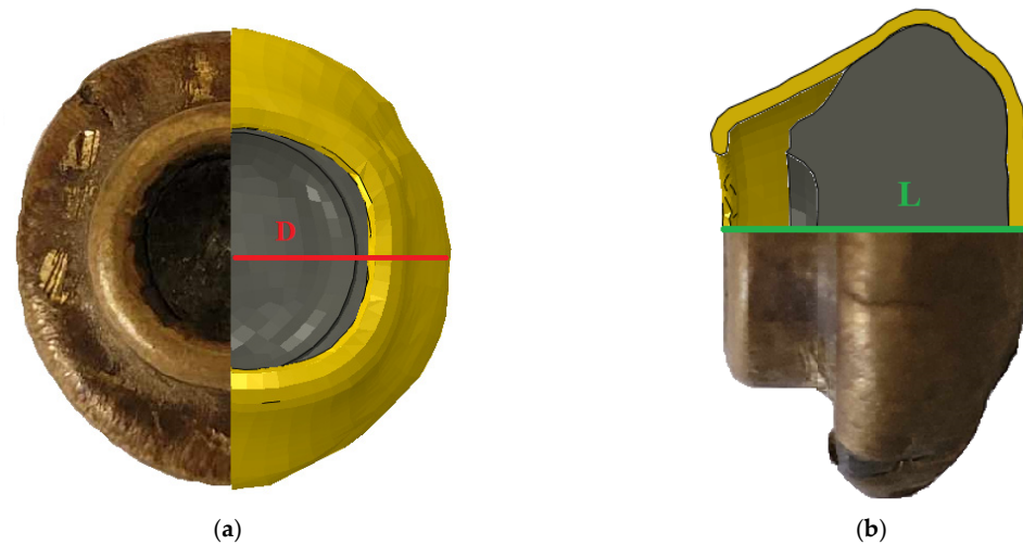
Figure 13. Comparison of projectile deformations after the ballistic tests and numerical tests: (a) rear side of projectile; and (b) side view of projectile.
