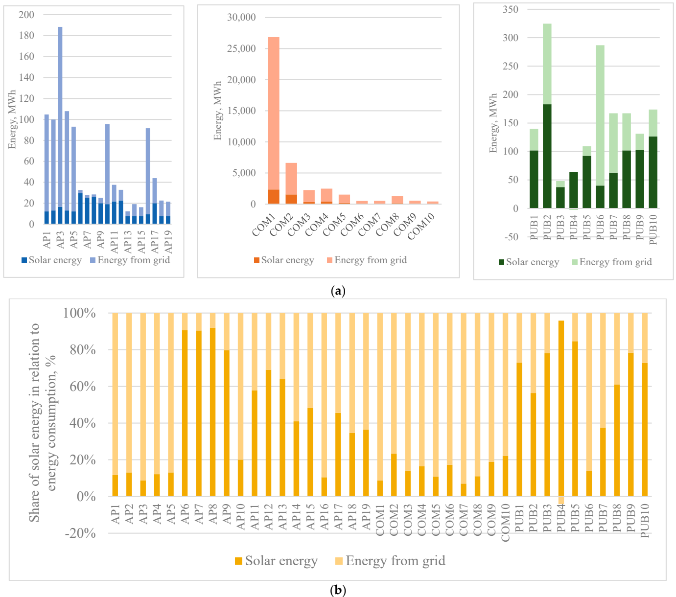
Figure 8. Amount (MWh) and share (%) of solar energy in relation to total energy consumption in buildings (done by authors). (a) Annual solar energy yields relative to the annual energy consumption in the building, MWh (done by authors). (b) Solar energy as a share of total energy consumption in the building, % (done by authors). Note: Light color represents amount of annual building consumption covered by solar energy and dark color shows remaining energy consumption taken from the grid.
