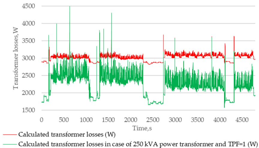
Figure 9. Loss comparison with smaller power transformer with good power quality.
