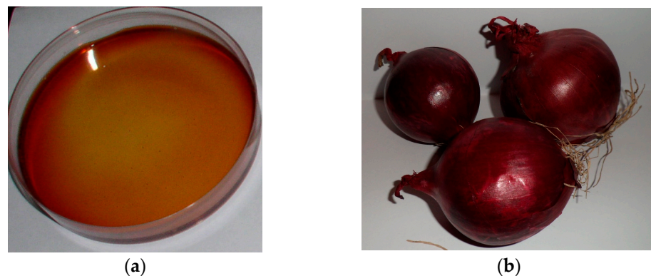
Figure 5. A photograph of red onion peel extract–gelatin-silver nitrate gel films in a Petri dish (a) and red onion bulbs (b).
