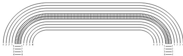
Fig. 1. Numbering of lines equidistant in the normal direction to the surfaces of the structure for the plane strain problem
