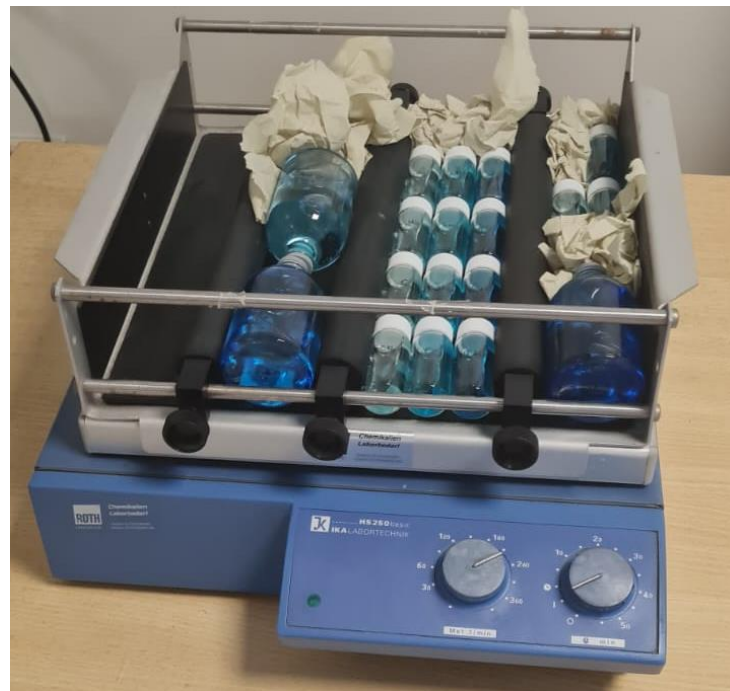
Fig. 8. IKA LABORTECHNIK HS250 basic shaker with a special mount to keep the vials in position
