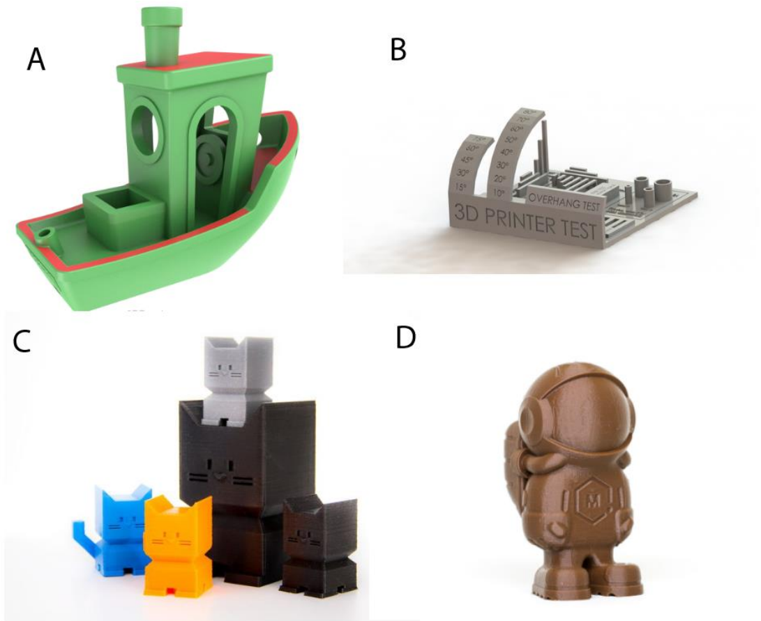
Fig 9. Different 3D printing test prints. A – Benchy; B- All in one; C – Cali Cat; D – Phil A. Ment
