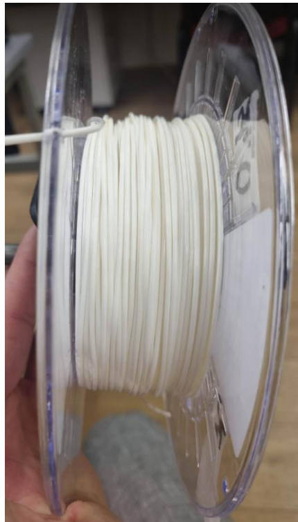
Fig 12. Example of the produced filament with \text{TiO}_2
