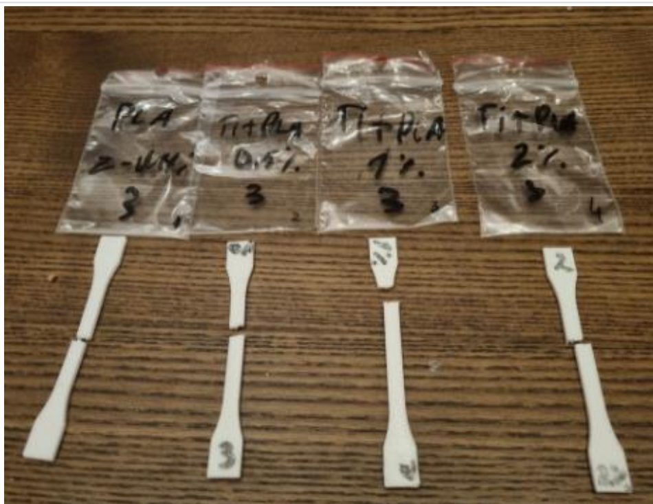
Fig 22. PLA +TiO 2 2 Gy Mechanical test results
