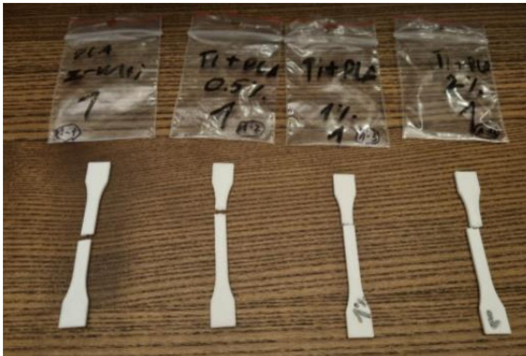
Fig 23. PLA +TiO 2 70 Gy Mechanical test results
