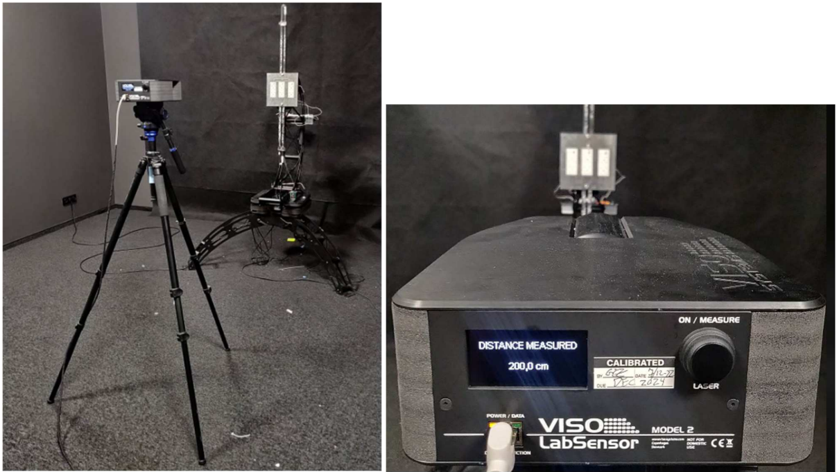
Fig. 26. UV-C source mounted on the goniometer and the set distance in the testing facility.
