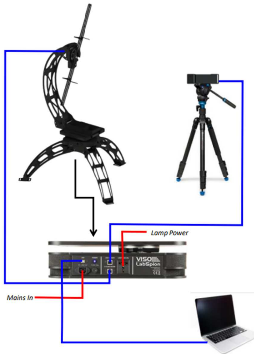
Fig. 18. Light measurement system connection scheme [88].
