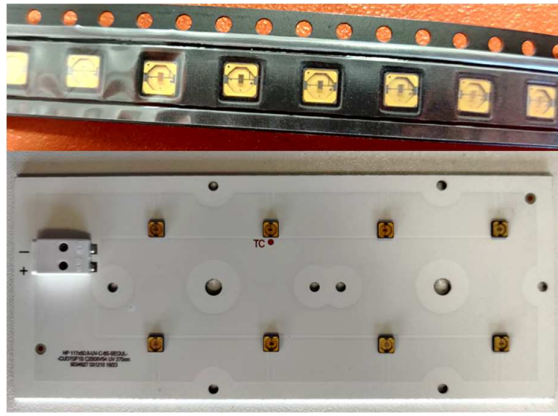
Fig. 14 Separate UV-C LED chips above and created LED module below.
