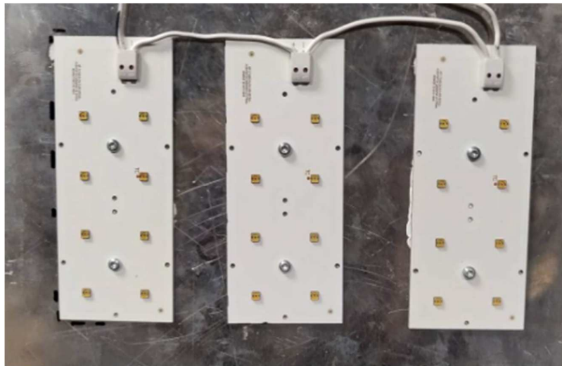
Fig. 25 LED modules mounted on the aluminium plate.
