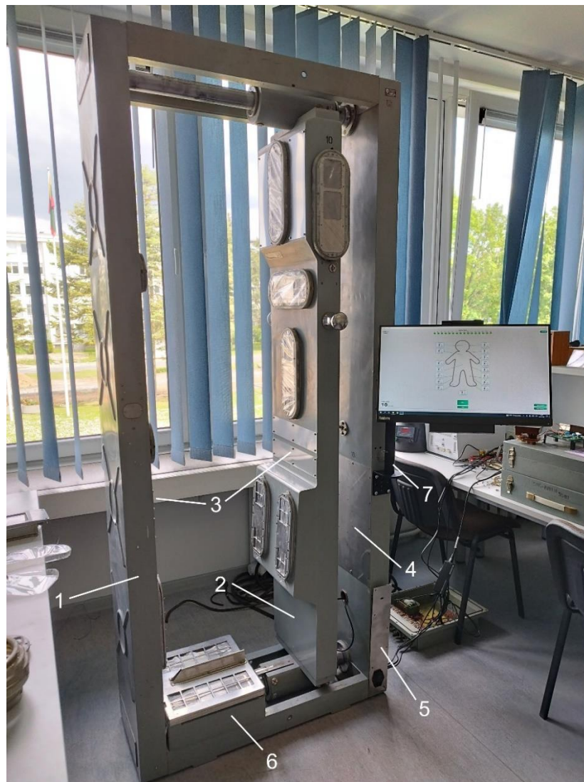
Fig. 24 Assembled modular radiometric measurement system (1 – left frame, 2 – middle frame, 3 – left and middle cavity, 4 – right cavity, 5 – bottom cavity, 6 – bottom module housing, 7 – monitor arm)
