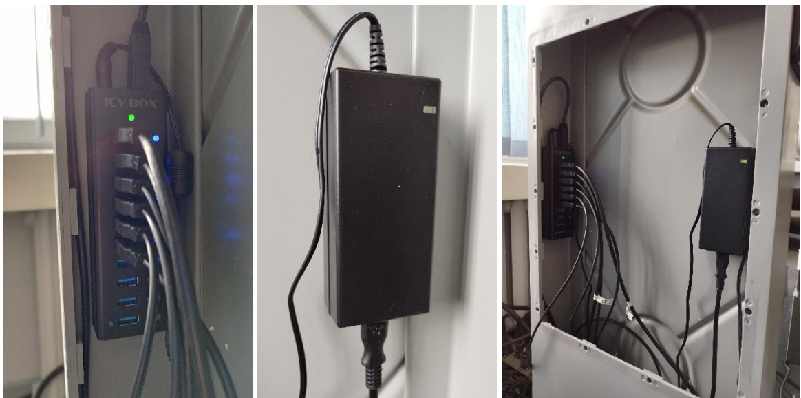
Fig. 23 ICY BOX USB hub (left), 5 Volt AC/DC converter (middle), component cavity (right)
