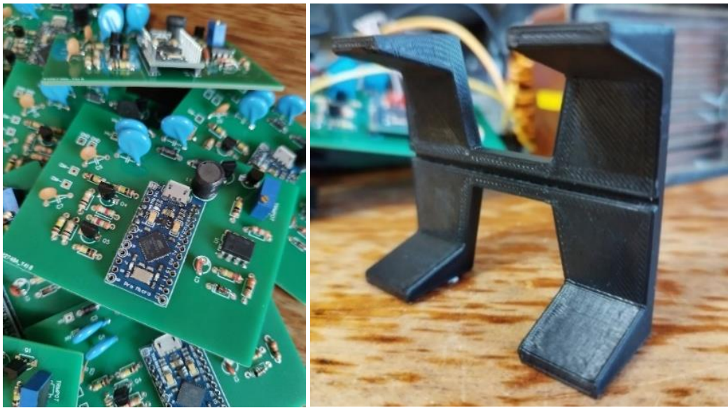
Fig. 13 Main Arduino-equipped circuit board (left) and board standoff (right)
