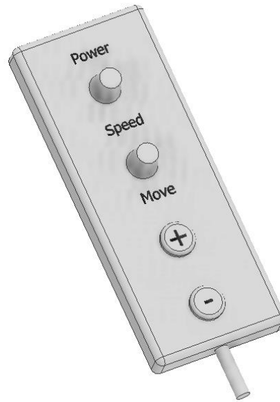
Fig. 35. Designed remote controller for the wearable assistance rehabilitation robot
