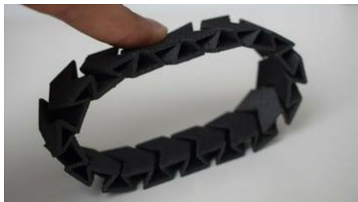
Fig. 19. Flexible carbon fiber reinforced part with TPU matrix with electrostatic resistance [14]
