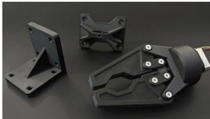
Fig. 18. High tensile strength parts 3D printed using lose carbon fiber reinforced nylon filament [14]
