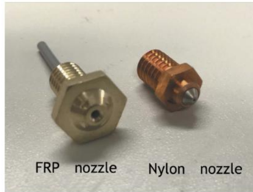
Fig. 20. Nozzles used for 3D printing CFRP composite structures [15]
