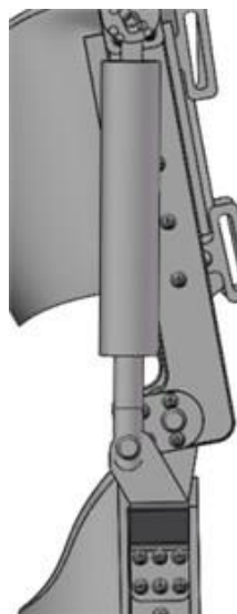
Fig. 10. Knee exoskeleton with a hydraulic cylinder as an actuator [14]
