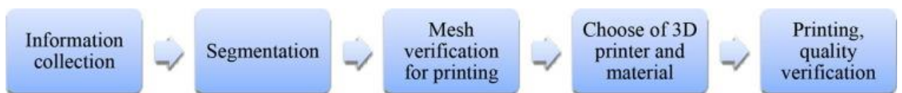
Fig. 13. 3D printing method [17]
