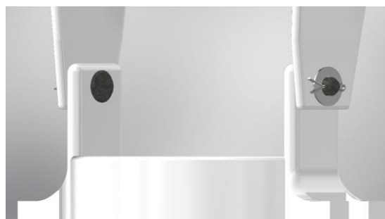
Fig. 29. Connection of top and lower exoskeleton parts
