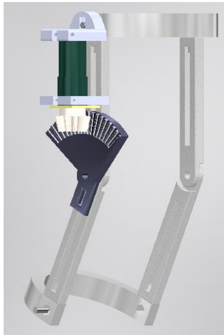
Fig. 33. Servo motor with bevel gear transmission as an actuator
