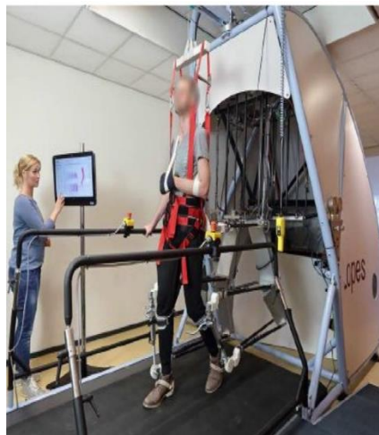
Fig. 11. LOPES exoskeleton which is manufactured by metal casting and CNC machining [15]
