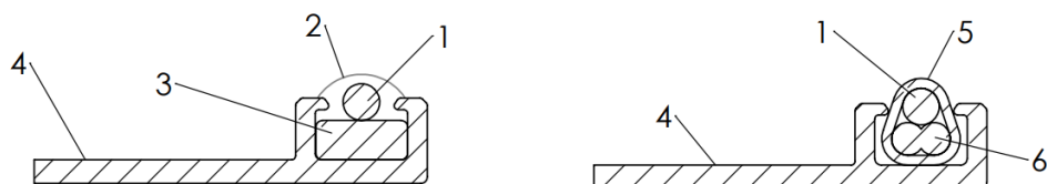
Fig. 31. Structures for piezo cable stabilization in aluminum profile, structure with silicone and rubber spacer (left), and structure with thermo tube and isolated cable with two wires used as a spacer (right). 1 – Piezo cable, 2 – Silicone layer, 3 – Rubber, 4 – Aluminum profile, 5 – Thermo tube, 6 – Isolated cable with two wires
