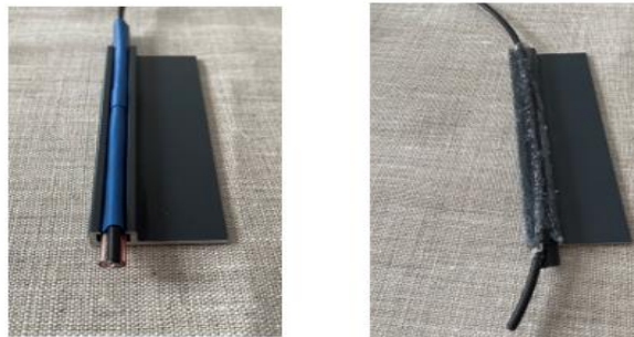
Fig. 36. Piezoelectric construction spacer material sample with thermo tube and two-wired cable (left) and another sample with rubber and silicone layer (right)
