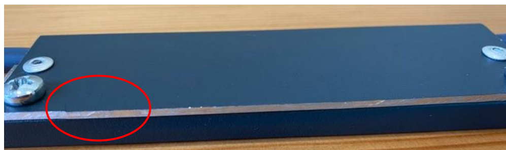
Fig. 48. Deformed top surface edge of the aluminum profile (marked red)
