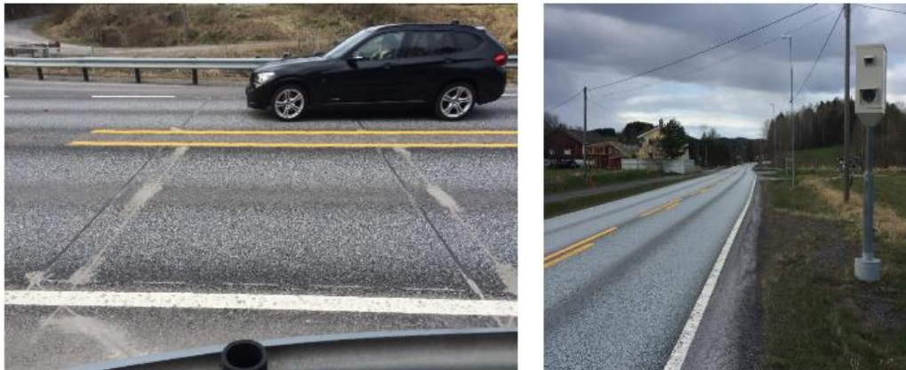
Fig. 19. Speed enforcement system of piezo cables and camera unit [21]
