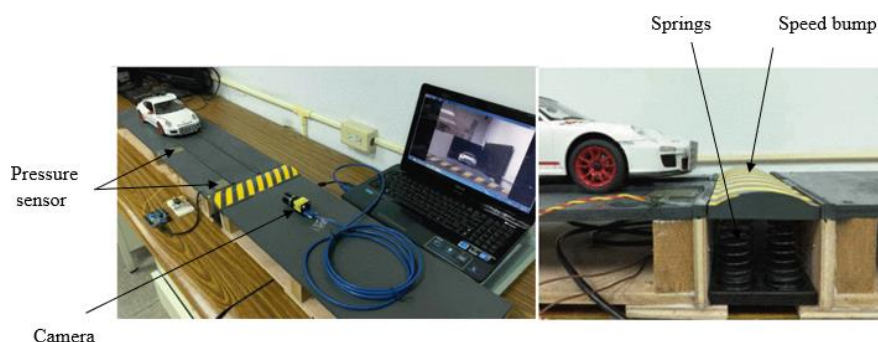
Fig. 3. The prototype of an adaptable speed bump with license plate recognition [10]
