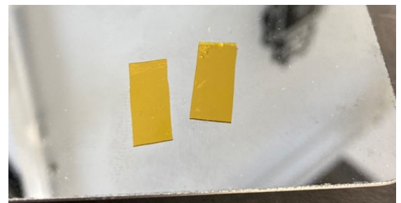
Fig. 44. Samples made out of Kapton tape
