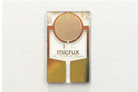
Fig. 10. Thin film Gold Inter Digitated Electrode produced by Micrux Technologies [13]
