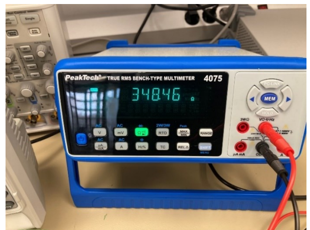
Fig. 66. Measuring resistance of strain gauge
