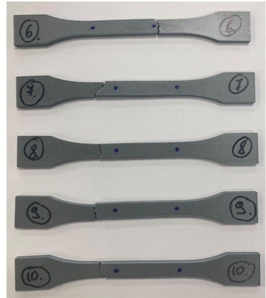
Fig. 54. Samples with strain gauge dummy after the disintegration
