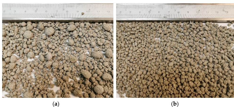
Figure 12. AA granules before sieving (a) and after sieving with a 4 mm sieve (b).
