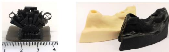
Figure 1. DLP 3D printed object of AESO/IBOMA (left) and 3D printed lower human jaw bone fragments of commercial resin (light) and AESO/THFMA resin (black) (right).
