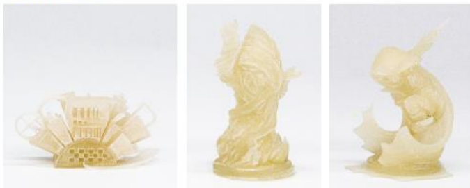
Figure 2. DLP 3D printed AESO-based composites: complex shape object of AS40/I60/XS5 (left) and action figures of AS40/I60/XSM5 (middle and right)
