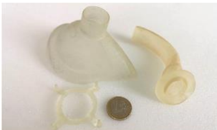
Figure 3. 3D printed medical fittings produced in 3D Creative by Zortrax Inkspire 3D printer.
