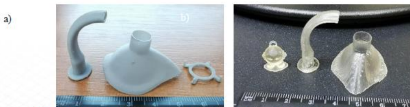
Figure 2. Reduced size 3D printed medical fittings of commercial resin Asiga PlasGray (a) and AESO-based resin (b) using Asiga Pico UV 3D printer at VU LRC
