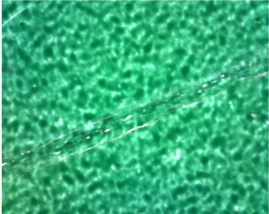
Fig. 3.5.1. Tinplate bended by 180 degrees.
