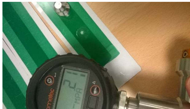
Fig. 3.2.4. Minimum force applied on two layer surface
