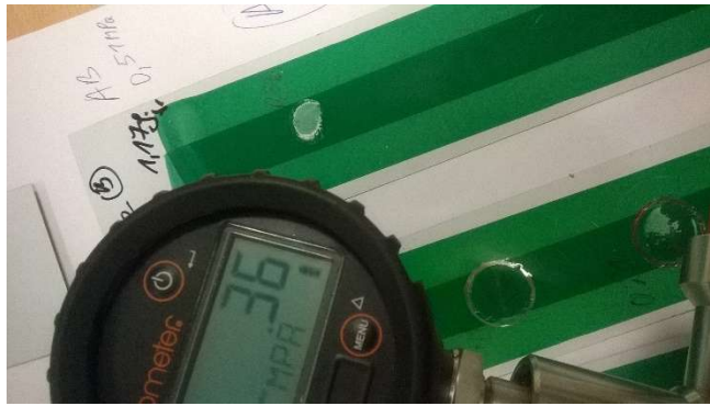
Fig. 3.2.6. Maximum force applied on a two layer surface The coating around the dolly was cut using the dolly cutter.
