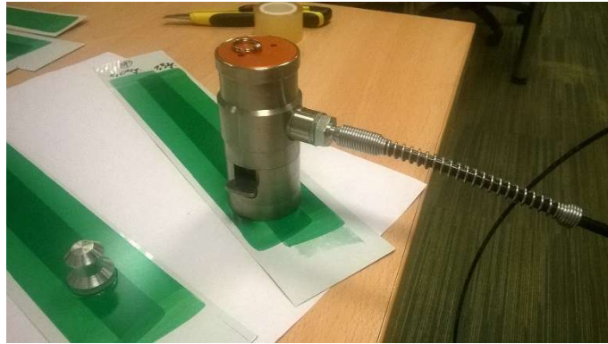
Fig. 3.2.3. The actuator placed over the dolly
