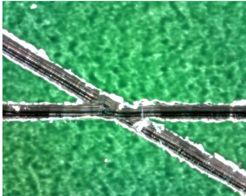
Fig. 3.4.2. Microscope result of X-cut test
