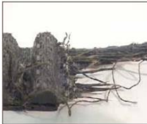
Figure 1.3.6 Shock load failure example
