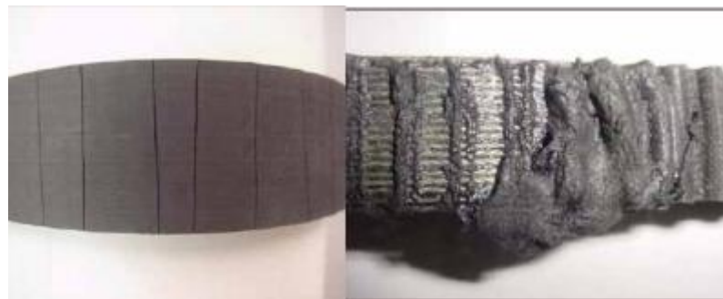
Figure 1.3.10 Timing belt reaction to high temperature
