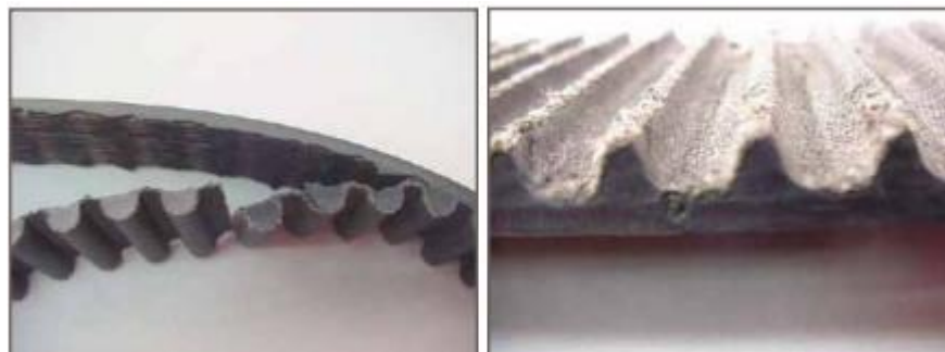
Figure 1.3.8 Low belt tension example
