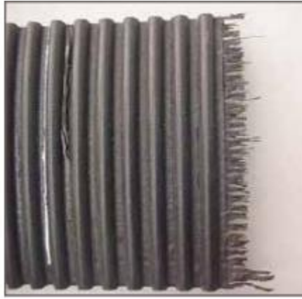
Figure 1.3.5 Crimp failure example
