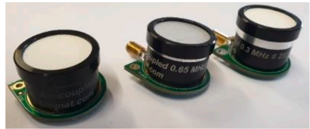
Fig. 1. Transducers used in experiments (left: 1 MHz, center: 650 kHz, right: 300 kHz center frequency).
