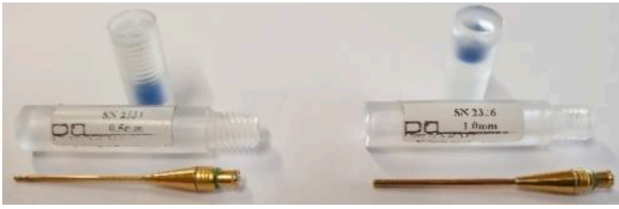
Fig. 3. Needle hydrophones used in the experiments (left: 0.5 mm, right: 1 mm).
