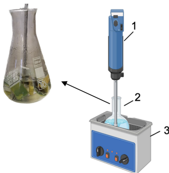
Figure 1. A laboratory-scale reactor was utilized in the study. 1: Overhead mixer. 2: Flask containing MLPW strips and aqueous nitric acid solution. 3: Ultrasonic bath. The Erlenmeyer flask provides an accurate representation of the experimental setup. The photograph of the flask highlights the necessity for a substantial volume of acid relative to the minimal weight of the pack.
