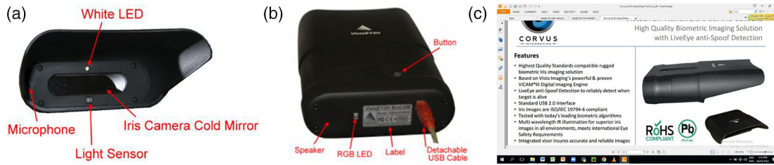
Figure 1. (a). The Camera's Front View. (b). The Camera's Back View. (c). The Camera's Side View.
