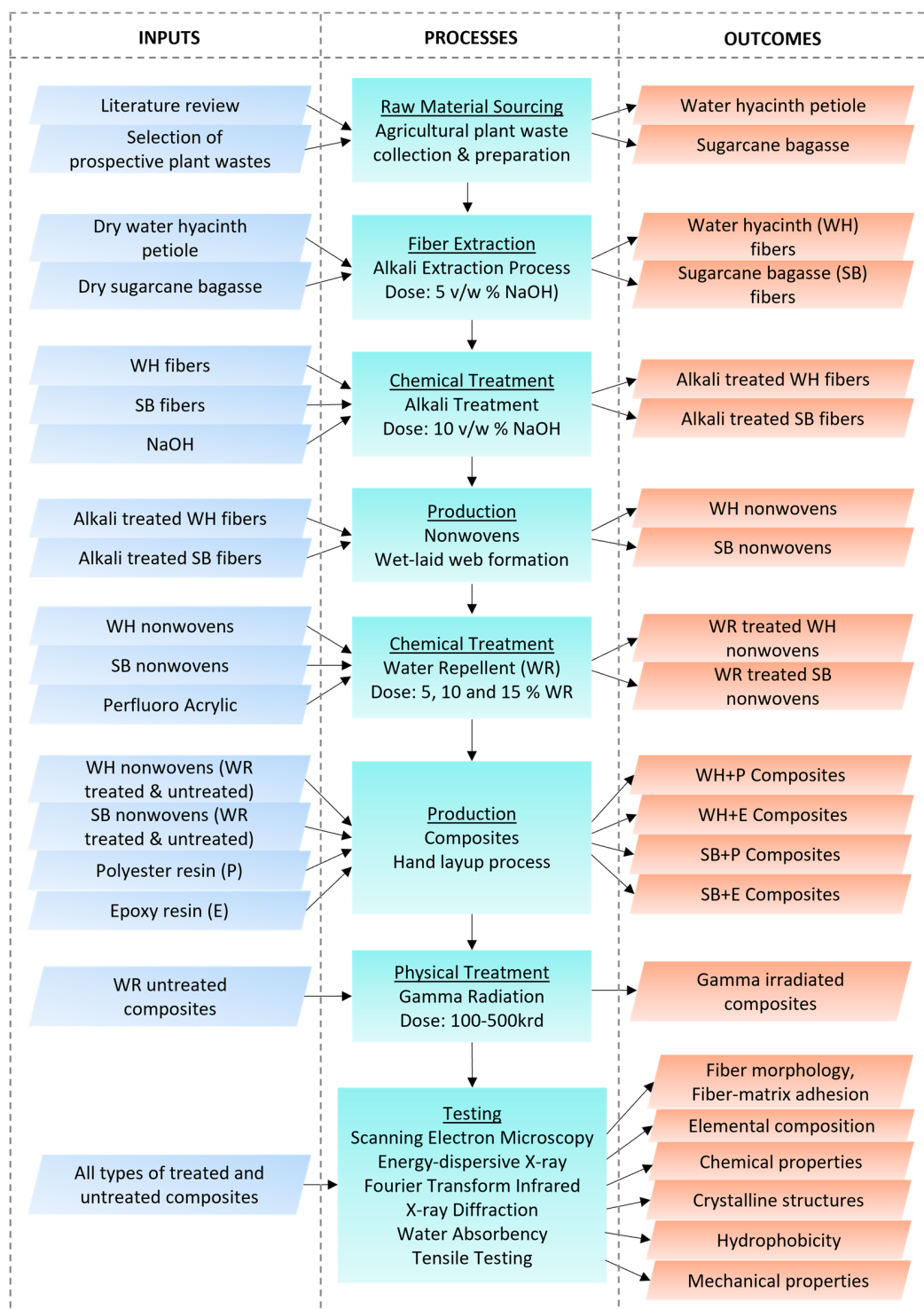
Figure 1. Experimental process scheme.
