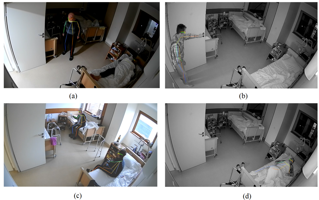
Figure 9. Examples of skeleton-based posture recognition in various ambient light conditions: (a) patient walks in a semi-lit environment; (b) patient walks during the night; (c) two patients sit in a fully-lit environment; (d) patient is lying down at night.
