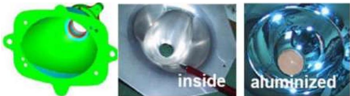
Figure 1.10. Reflective surface of the headlight [18]
