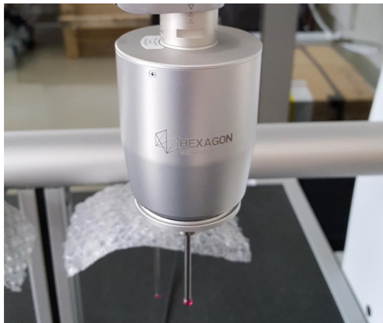
Figure 3.12. Measuring probe of the CMM machine
