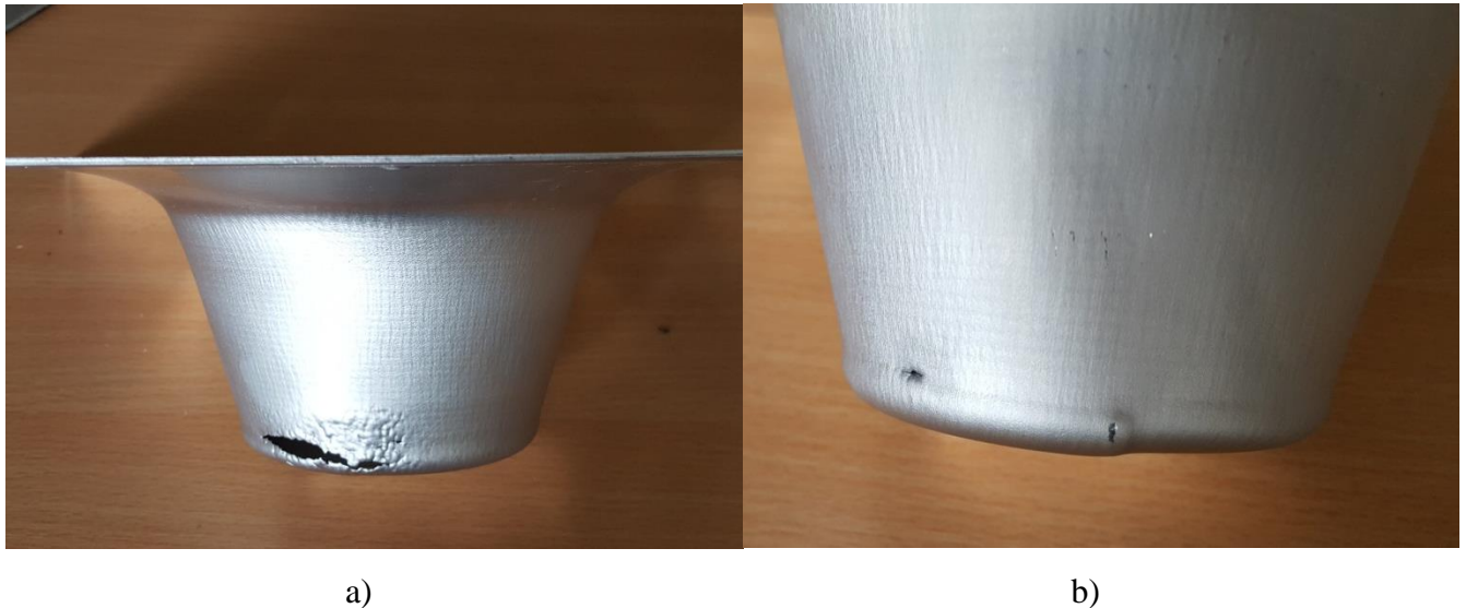
Figure 3.5. Fractured cones with contact angle of 74^\circ at different depths: a) fracture at 45 mm, b) fracture at 75 mm
