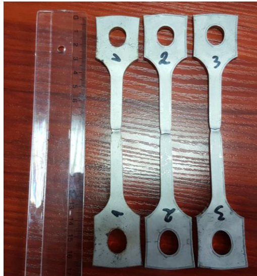
Fig. 3.3 Virgin plates after fracture
