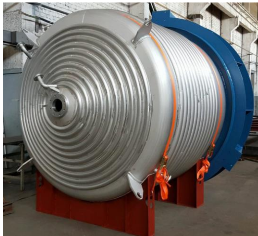
Fig. 5.1 Manufactured vertical conical pressure vessel with half-pipe coil
