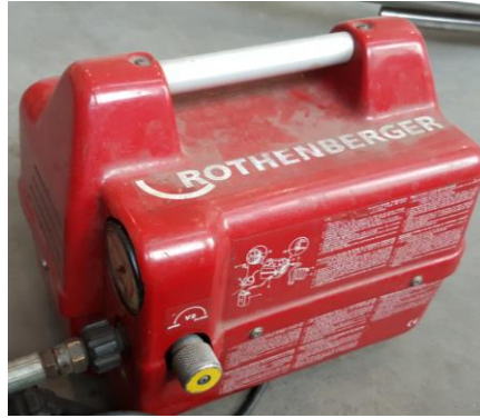
Fig. 5.2 “Rothenberger RP Pro II” pump used for pressure test
