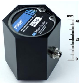
Fig. 1.5 Piezoelectric vibration energy harvester from MicroStrain ® [21]
