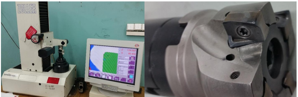
Fig. 7.3 Blunt tool measuring device Zoller Smile v300
