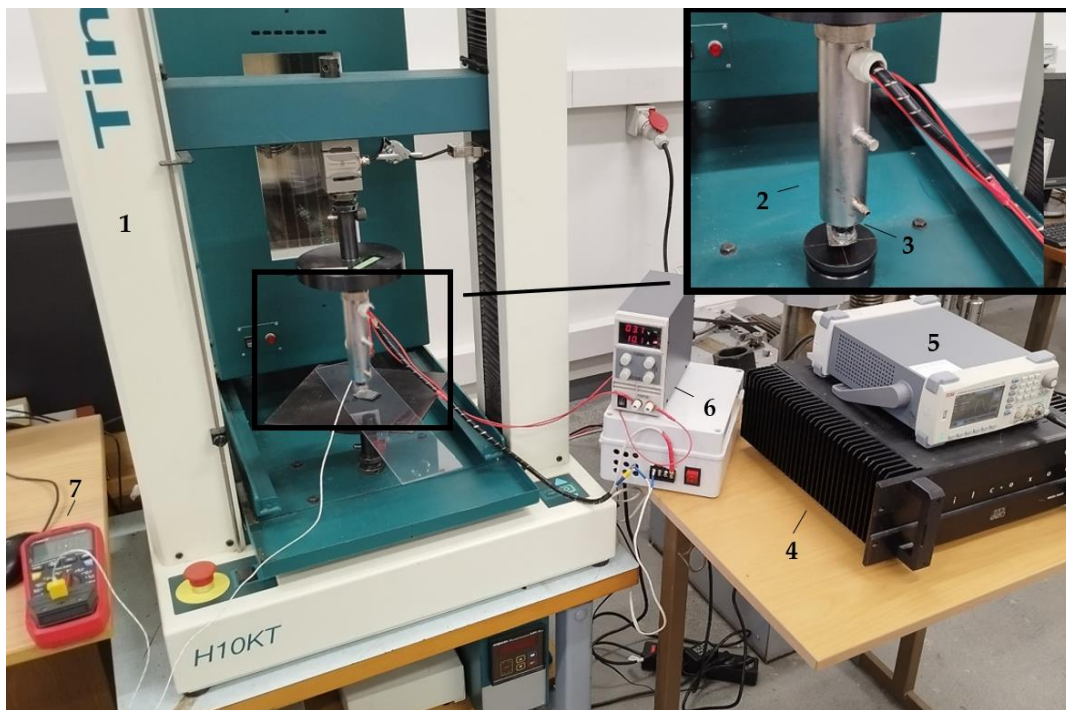
Figure 7. Microstructure forming equipment: 1—Tensile test machine H10KT (Tinius Olsen, Horsham, JAV), 2—magnetostrictor, 3—forming grid, 4—amplifier PA8HF (Wilcoxon, Gamlingay, UK), 5—signal generator UTG2025A (UNI-T, Hong Kong, China), 6—power source KPS3010D (wanptek, Shen Zhen, China), 7—thermometer UT161D (UNI-T, Hong Kong, China).
