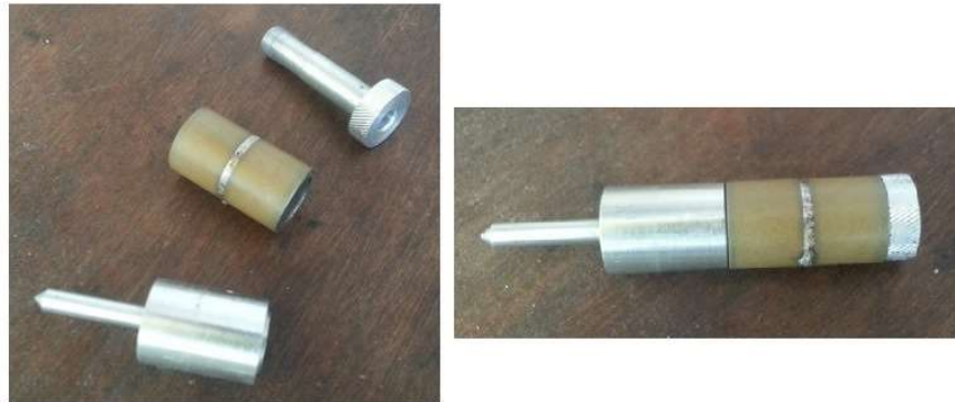
Figure 2.4 Individual parts and assembly of the nozzle
