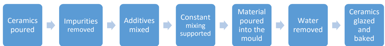
Figure 3.9 Sequence scheme for manufacturing
