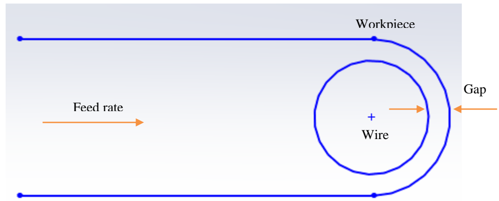
Fig. 2.7. Gap size and feed rate
