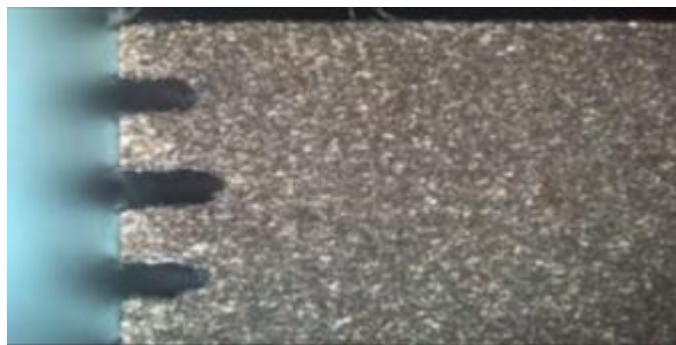
Fig. 2.8. Broken wire and small cutting line in titanium machining due to low flushing pressure [26]
