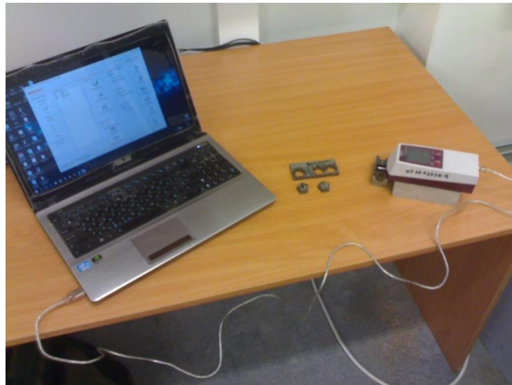
Fig. 4.14. SurfTest SJ-210 device connected to laptop
