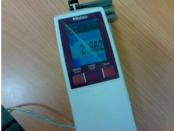
Fig. 4.13. SurfTest SJ-210 device showing the results
