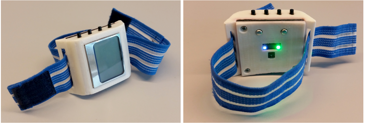
Figure 2.12: The wearable PPG wearable device: front (left) and back (right)
