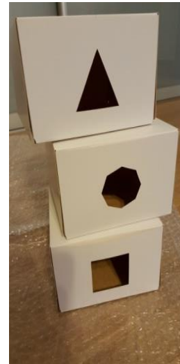
Fig. 4 Test samples with three different cuttings shapes (square, triangle and octagon) in the front package wall
