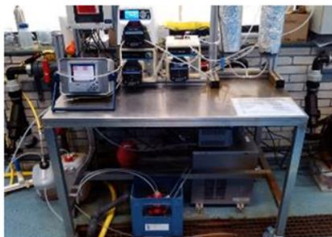
Fig. 7. Scheme of a filter column filled to form BioFeO on sand and glass foam and the photo of the set-up
