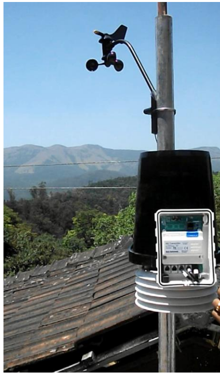
Figure 11 Installed wireless weather monitoring station [20]
