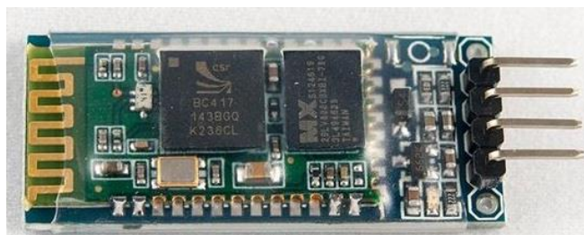
29 pav. HC – 06 Bluetooth modulis[14]
