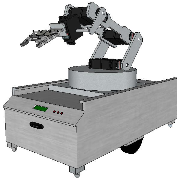
Figure 2.2 Line tracing robot with robotic arm
