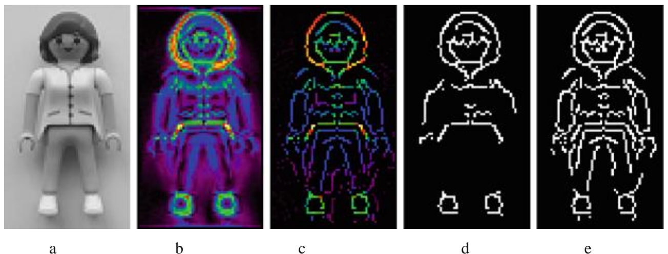
Figure 26 An example of the Canny operator is shown: a) intensity image; b) output of gradient filter in pseudo color, the gradient magnitude increases in the following order: black – violet – blue –green – red – yellow – white; c) gradient after non-maximum suppression in pseudo color; d) detected edges with high thresholds; e) detected edges with low thresholds [40]
